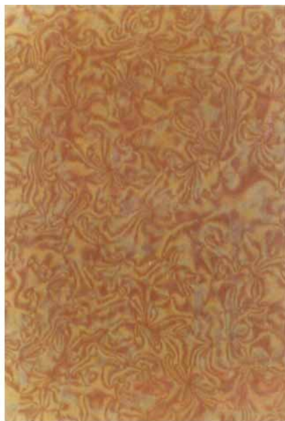
Figure 5. Top: fan texture of the smectic I phase of ATT 10 at 145°C ( \times 162 ). Bottom: smectic I schlieren texture of ATT 12 at 139°C ( \times 162 ).
